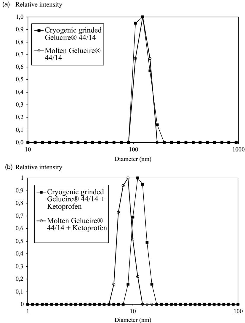
Fig. 5. Droplet size distribution of molten or cryogenic grinded Gelucire® 44/14 alone (a) and with ketoprofen (b).
