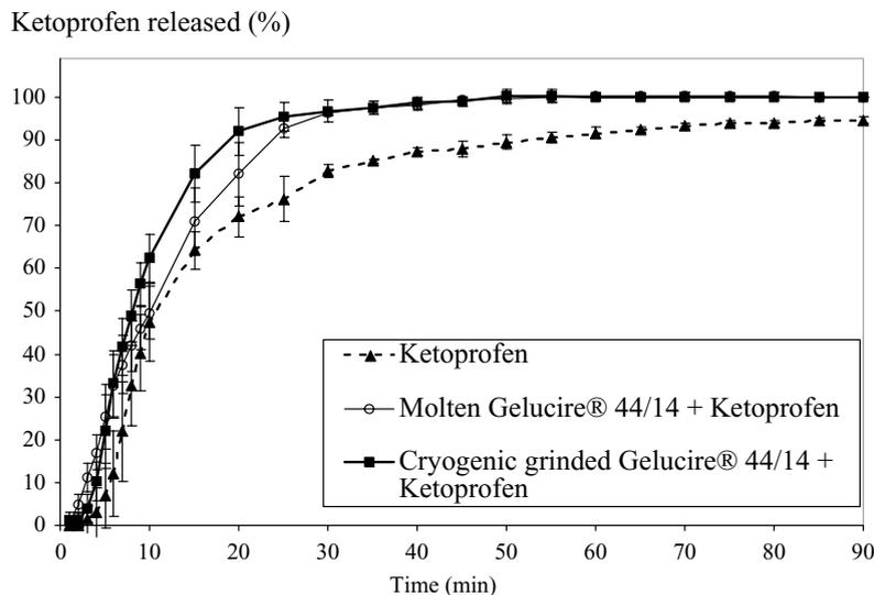
Fig. 6. Dissolution profiles obtained with ketoprofen (Topfena<sup>®</sup> capsules), molten Gelucire<sup>®</sup> 44/14/ketoprofen mixture and cryogenic grinded Gelucire<sup>®</sup> 44/14/ketoprofen mixture.
