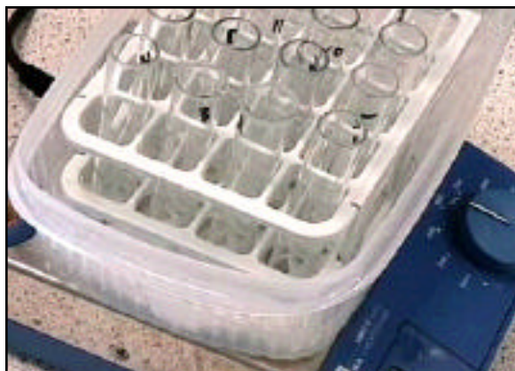
Figure 1. Arrangement of ice-water bath over a magnetic stirrer for treatment of samples with 2 M KOH and dissolution of RS.
