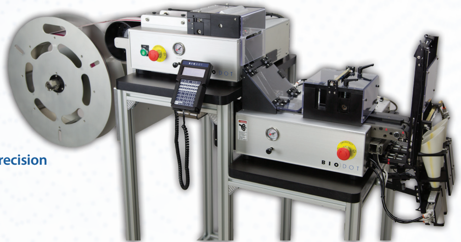
Cutter with roll feed and bottle collection
