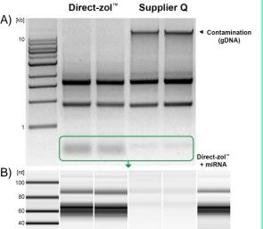
High quality broad range RNA is purified with the Direct-zol™ RNA MiniPrep. (A) DNA-free RNA purified from human epithelial cells using the Direct-zol™ RNA MiniPrep compared to a DNA containing preparation from Supplier Q (1% agarose/TAE). (B) Small RNAs are effectively recovered with the Direct-zol<sup>™</sup> procedure while absent in Supplier Q preparations (Agilent Bioanalyzer 2100, Small RNA Chip data shown).
