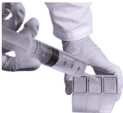
Figure 5. Filling the feeding compartment.
